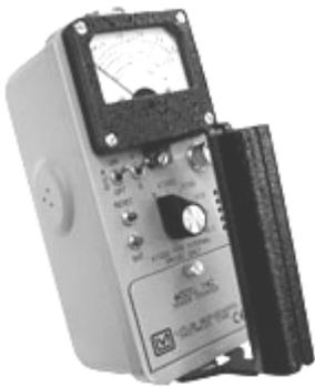
The Model 14C is a rugged splash-proof portable survey instrument that operates on two standard "D" cell alkaline batteries. The instrument features a regulated high-voltage power supply set at 900 volts and provides five linear ranges for measurement from 0 to 2000 mR/hr.
