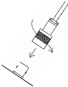
Connect one end of a detector cable to the detector by firmly pushing the connectors together while twisting clockwise a quarter of a turn. Repeat the process in the same manner with the other end of the cable and in the instrument.
