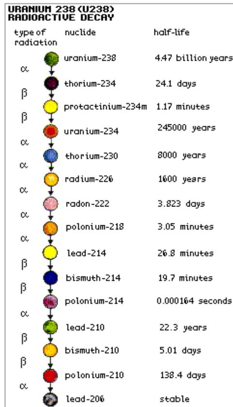
All uranium atoms are mildly radioactive. The following figure for uranium-238 shows the series of different radioisotopes it becomes as it decays, the type of radiation given off at each step and the half-life of each step on the way to stable, non-radioactive lead-206. The shorter-lived each kind of radioisotope, the more radiation it emits per unit mass. Much of the natural radioactivity in rocks and soil comes from this decay chain.
