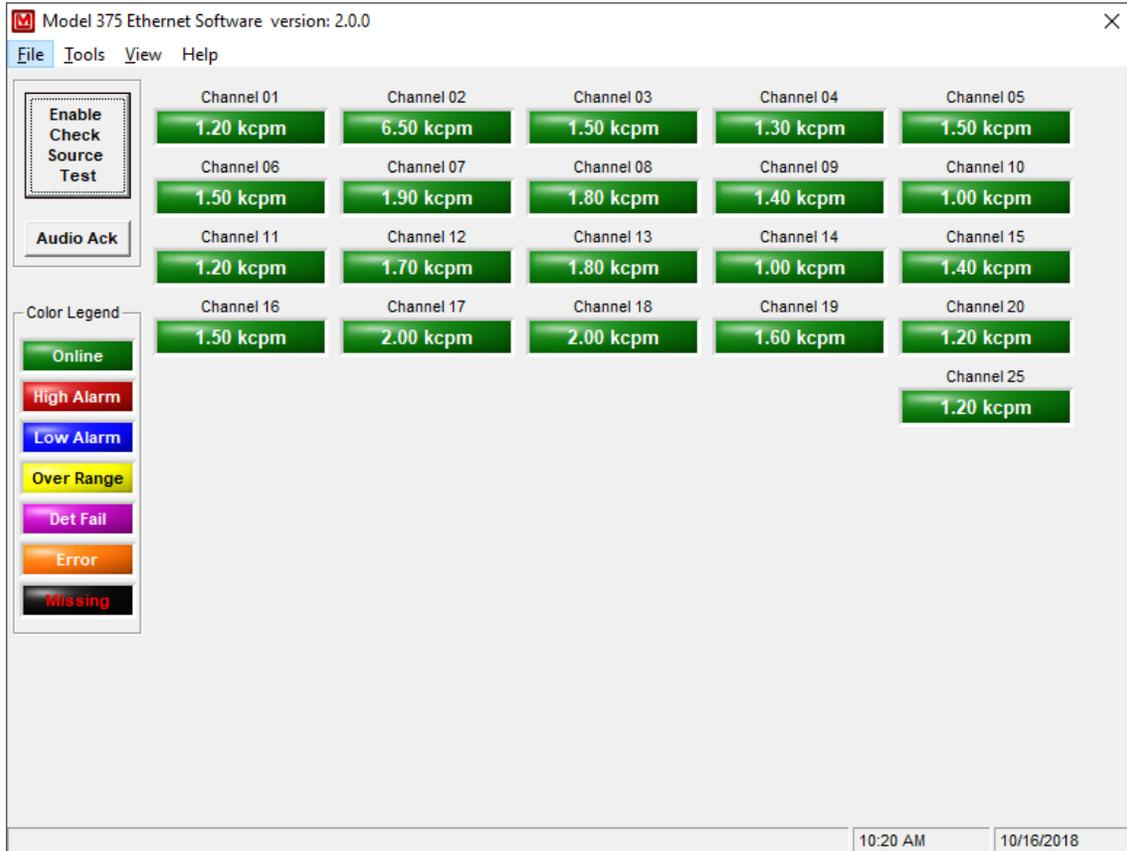
The main window displays reading boxes for all enabled Model 375s along with their status, units, and caption. Left-clicking on the channel will open a web browser to the camera if enabled. Right-clicking on the channel name will display the last image and alarm information that has occurred since the program was running. Holding the mouse over the channel name will display a tool tip with the user-defined comment.
