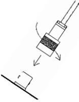
Connect one end of the cable provided to the detector by firmly pushing the connector together while twisting clockwise one quarter of a turn until latched. Repeat the process in the same manner with the other end of the cable and the instrument.
