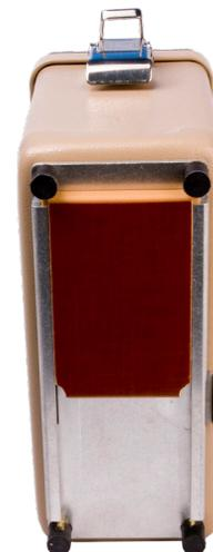
*rear view showing the retractable beta shield*
