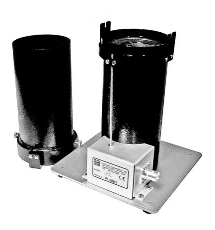
Model 182 Radon Flask Counter – open
