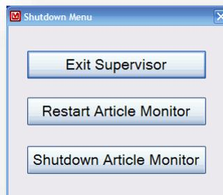
Exit Supervisor – Closes the Supervisor application and provides access to the Windows XP Embedded environment. This is necessary for performing software updates, configuring Windows settings such as printing or networking, or to provide access to the data files. A confirmation window will be displayed before the Supervisor application is closed.
