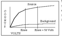
**Scintillators**: Set the DISC for 10 millivolts. Plot background and source counts versus HV to produce a plateau graph similar to the one in the figure. Adjust the HV to 25-50 volts above the knee or start of the plateau. This provides the most stable operating point for the detector.
