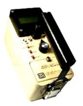
he Model 2241 is a portable microprocessor-based digital scaler/ ratemeter designed for use with scintillation, Geiger-Mueller (GM), and proportional type detectors to measure ionizing radiation. Data is presented on a four-digit (six digits in the Scaler mode) Liquid Crystal Display (LCD) with moving decimal point. A threeposition switch labeled OFF/RATEMETER/SCALER selects the desired operating mode for the instrument.
