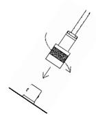
The detector operating voltage (HV) is supplied to the detector via the detector input connector. A mild electric shock may occur if you make contact with the center pin of the input connector. Switch the Model 2360 to the "OFF" position before connecting or disconnecting the cable or detector.
