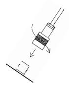
The detector cable can be a source of problems. Test the detector cable by bending or flexing either end of the cable and checking for an increase of counts detected. Replace the cable if increases in the rate of counts are detected.
