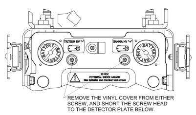
Figure A-1. Discharging Gamma Wall Voltage.
