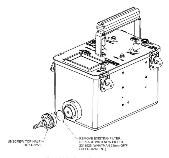
Figure 5-5. Particulate Filter Replacement.
