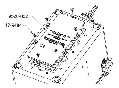
Figure 5-1. Battery Lid Removal
