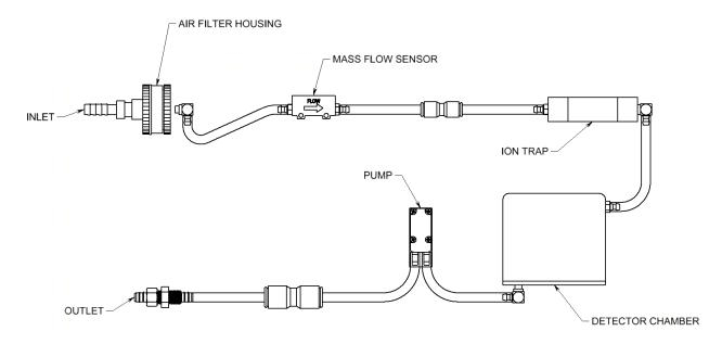
Figure 4-3. Air Flow Diagram.
