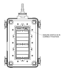
Figure 5-2. Battery Compartment.
