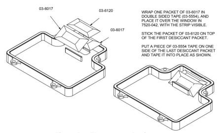
Figure 5-4. Electrometer Desiccant.
