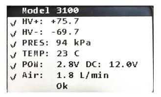
Figure 2-2. First Check Display Screen.
