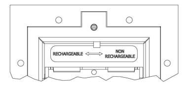
Figure 5-3. Battery Selection Switch
