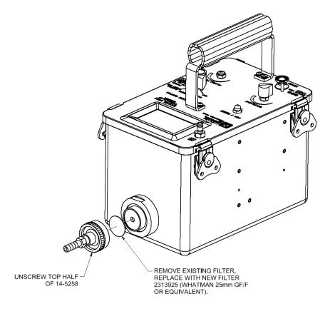
Figure 4-2. Particulate Filter.
