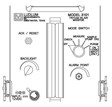
Figure 2-1. Identification of Controls.
