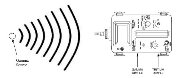
Figure A-2. Calibration Setup.
