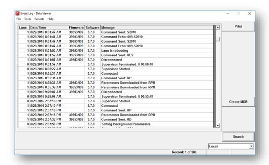
The main screen consists of a grid displaying the events recorded during the search query when viewing event log data.
