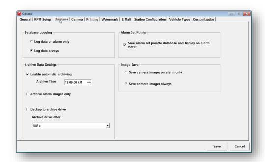
**Database Logging:** Sets how the occupancies are logged to the database. The occupancy data can be logged for every vehicle that passes through the RPM or only for vehicles that alarm. Alarms include both radiation and over-speed.
