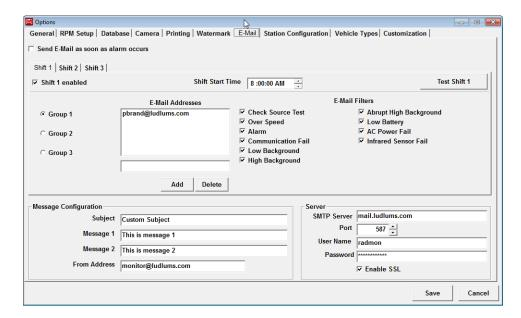
The E-Mail tab configures the Supervisor to send e-mail alerts when an RPM is alarming. There are three shifts that can be defined, each with their own set of six e-mail addresses. If a camera is enabled, then the image will be attached to the email. The image must be captured before the end of the occupancy to be included in the email. This means that triggering the camera on the exit of the occupancy with a delay time greater than 0 will not have the camera image attached.
