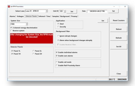
**System Size:** Sets the detector configuration. Typically, this parameter will never have to be changed. The system size is determined by the total cubic inches of the detector panels. Refer to the RPM calibration procedure for information on how to set these values properly. After changing the high voltage, the RPM should be rebooted.
