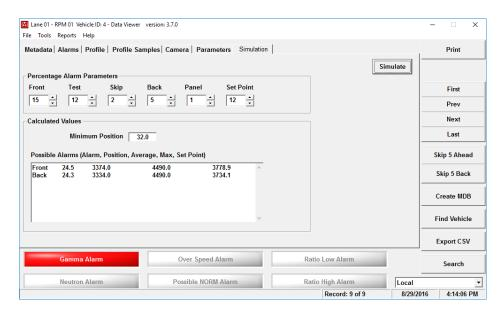
The Simulation tab can be used to modify the percentage alarm parameters and retest the vehicle for a percent alarm. Adjust the samples as desired, and click the Simulate button. The Minimum position of the alarm and the locations of possible alarms are calculated based on the current records' profile data.
