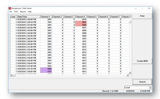
The main screen consists of a grid displaying the background readings recorded for all active RPMs when viewing background data. High background readings are colored with red, while low background readings are colored in purple.
