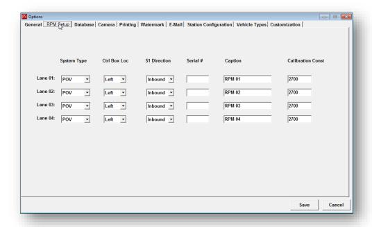
**RPM System Type:** Set the type of occupancies the lane will have. The choices are car, truck, or rail.
