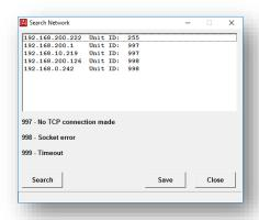
Click the Search button to begin searching for RPMs. When all available RPMs have been found, click the Save button. As each RPM is found, the Supervisor software retrieves its unit ID and displays it next to the IP Address. The Supervisor software displays several codes when retrieving the unit ID if a problem occurs. They are:
