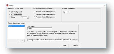
**Minimum Graph Scale:** Specifies the minimum graph scale for the Y-Axis on the profile graphs.
