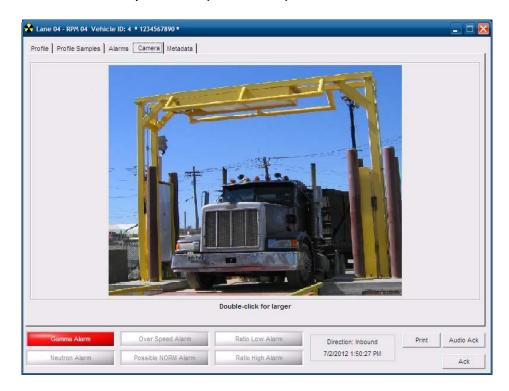
The Gamma Alarm (shown in red) indicates the presence of gamma radiation in excess of the sigma level set points. This alarm does not indicate the energy level or discriminate on the type of gamma radiation, just that the level is high and should be investigated further.
