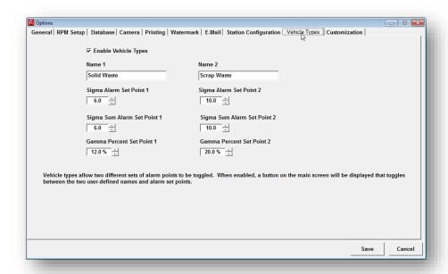
When enabled, this option allows two different alarm set points to be used depending on the type of vehicle. A button on the main screen toggles between the two sets of alarm parameters. The sigma set point applies to all detectors.
