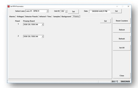
The Preamp tab is used to set the type of detector preamp that is installed. This should only be changed under the supervisor of an LMI technician.
