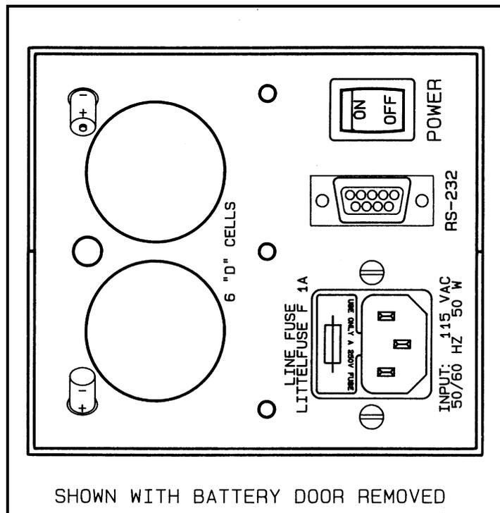
**Figure 5 – Model 52 Electronics Bottom View**
