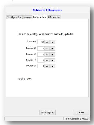
The isotopic mix is used to create a weighted average efficiency during monitoring cycles. Up to five isotopes may be used, which are defined in the Sources tab. The percentages must add up to 100%. The isotope names default to Source-1, Source-2, Source-3, Source-4, and Source-5 but will be updated to reflect the isotope names defined in the Sources tab.
