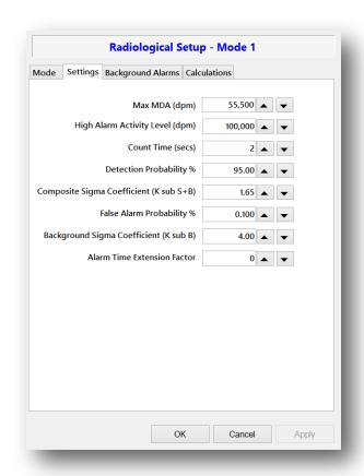
Max MDA – Sets the Mode 1 maximum MDA value. If the calculated MDA is greater than this value, a high background is posted. This value is set in specified activity units and is automatically converted when changed. The default value is 675 Bq.
