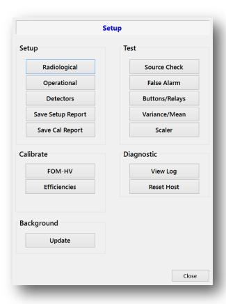
Radiological – Sets up the counting mode and its parameters, isotopic mix, occupancy mode, and units of measurement.
