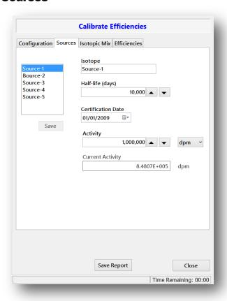
Up to five sources can be used in determining the efficiency. For each source, the half-life, certification date, and activity can be set. The current activity is automatically determined based on the data entered for the source and the current system time.
