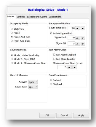
The Radiological Setup screen (see further explanation on following pages) provides access to the various parameters and options that control the counting modes, occupancy modes, isotopic mix, background alarm set points, and units of measure. The title indicates the current counting mode.
