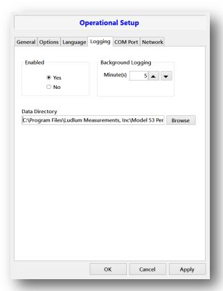
The Logging screen is used to set whether data logging is enabled, the directory where the data will be logged, and how often to log the background readings. When logging is disabled, no data will be saved to the scan, background, and system event logs.
