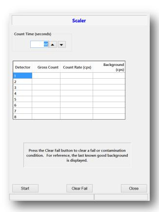
Once the contamination has been cleaned off the detectors or the cause of the fail has been corrected, take a scaler count to verify that the background values have returned to normal. If the background has returned to normal for all detectors, click Clear Fail to clear the fail condition and exit back to the main screen. A residual contamination check will be automatically performed followed by a background update if no contamination is detected.
