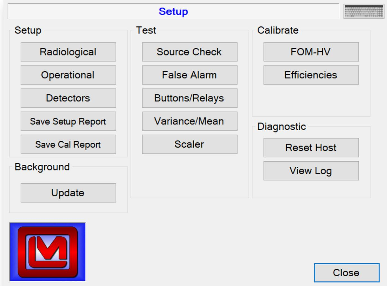
Radiological – set up the counting mode and its parameters, isotopic mix, and unit of measurements.
