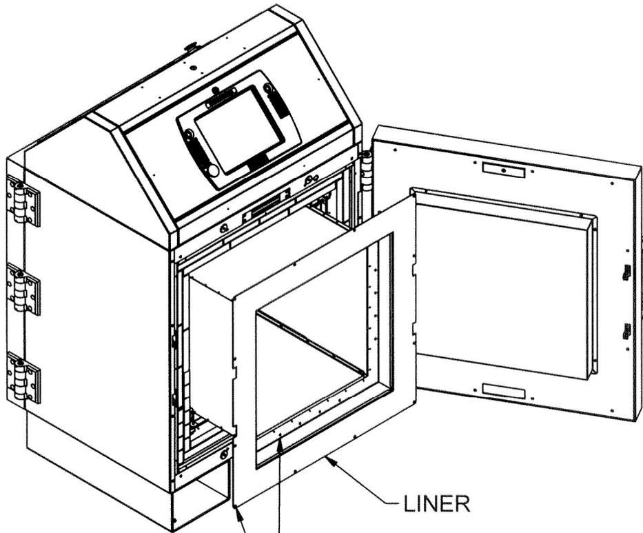
TO LOAD LEAD REMOVE THE OUTER AND INNER SCREWS TO ACCESS THE LEAD HOLDING AREA.
