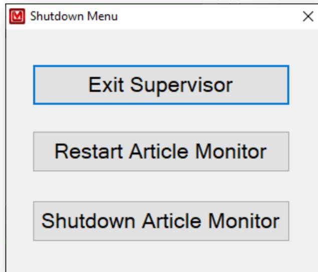
Exit Supervisor – Closes the Supervisor application and provides access to the operating system environment. This is necessary for performing software updates, configuring Windows settings such as printing or networking, or to provide access to the data files. A confirmation window will be displayed before the Supervisor application is closed.
