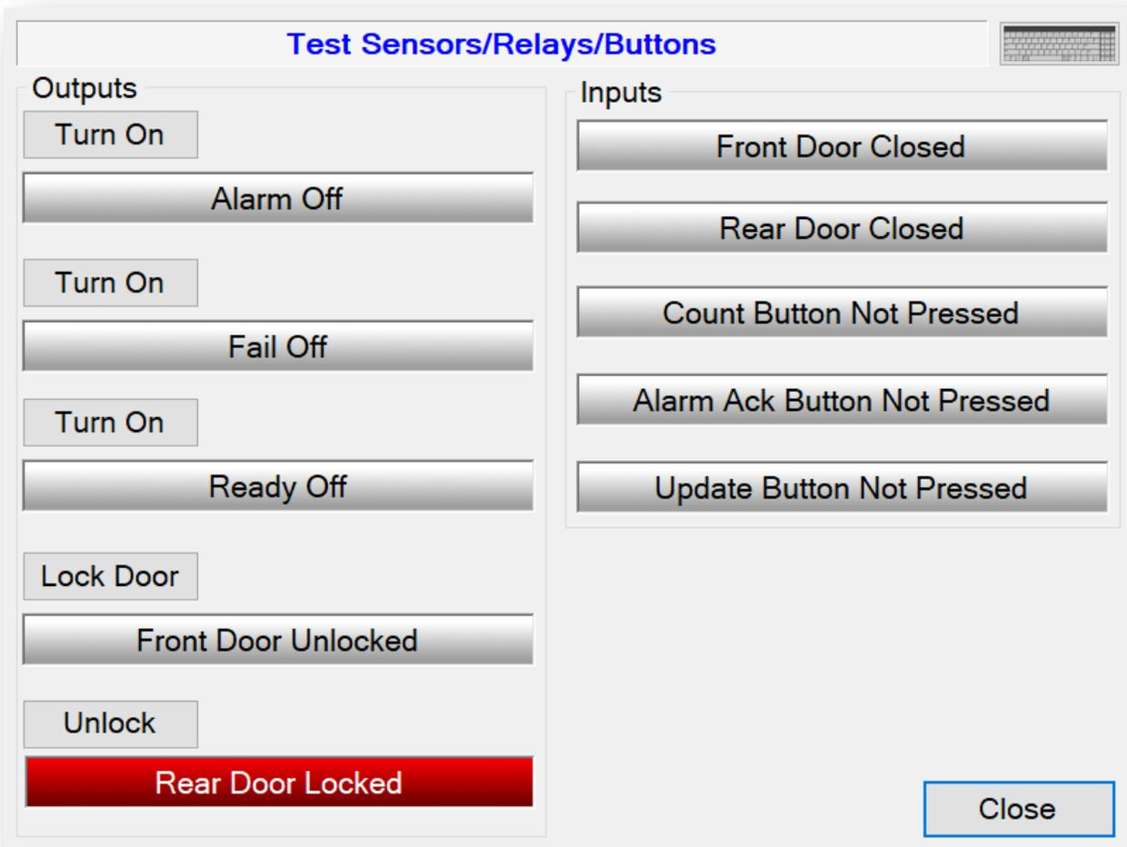
The outputs include the lights in the stack, relays, and door locks. The inputs include the door sensors and pushbuttons. Click on the buttons to turn on/off the lights/relays or lock/unlock the doors. When a pushbutton is pressed, the indicator should light up to indicate the button was read successfully. The article monitor should be taken out of service if any button, sensor, or light fails to respond correctly.
