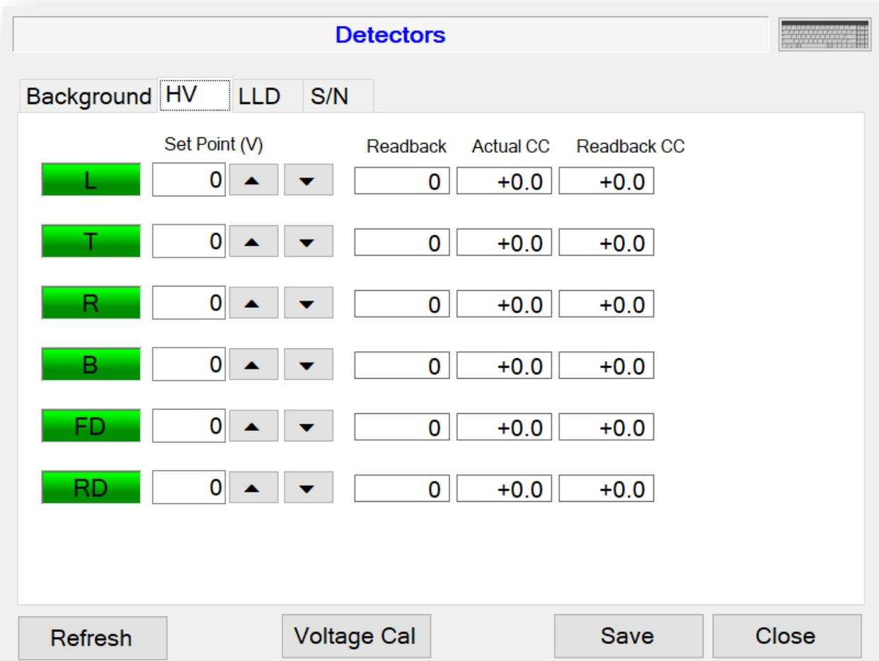
The HV screen displays the current high-voltage set point and calibration constants for each detector. High voltage is typically set using the FOM-HV screen. Read-back voltage is the value from the A/D converter. There are two calibration constants associated with the high voltage. The Actual calibration constant is used to calibrate the high-voltage output while the read-back
